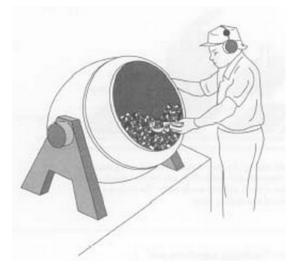
Towards the end of the process, grains of sugar are added to the spinning machine. It is this granular sugar that gives the jelly beans their hard outer shell. Finally, hot syrup and wax are added to the spinning machine to give the jelly beans their final polished, glossy look.
