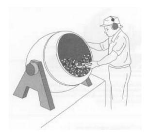
Towards the end of the process, grains of sugar are added to the spinning machine. It is this granular sugar that gives the jelly beans their hard outer shell. Finally, hot syrup and wax are added to the spinning machine to give the jelly beans their final polished, glossy look.
